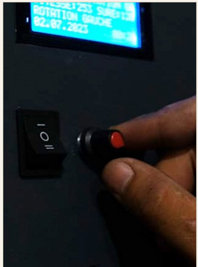
10B · FINE-SETTING THE ROTATION SPEED ON THE RED KNOB
