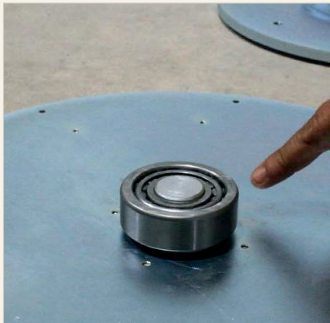
2A-II · CHECK THAT THE BEARING SITS FULLY HOME
