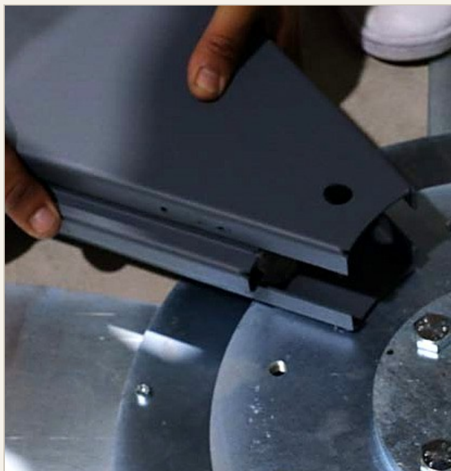
5B·I · A MALE-FEMALE PANEL OFFERED UP TO THE HUB
