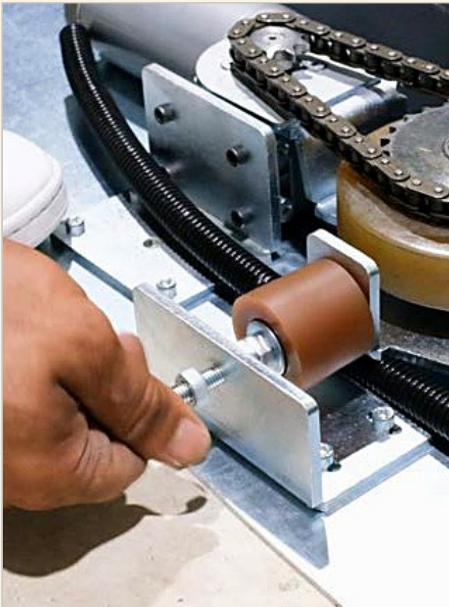
6A·I · THE STOP PRESSED HOME AGAINST THE PANEL WALL
