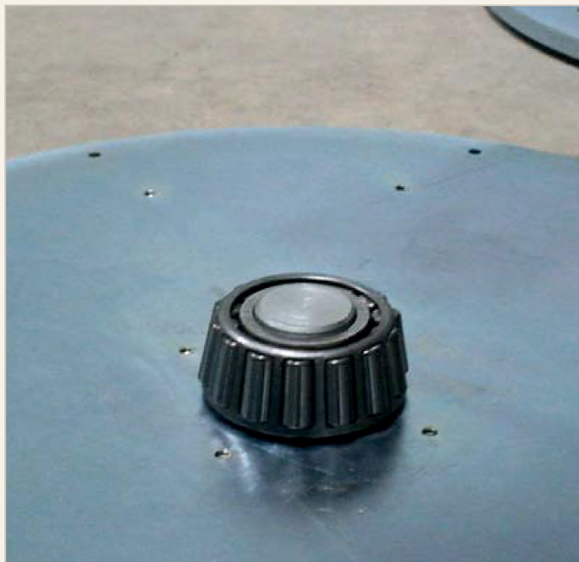
2A-I · THE TAPERED BEARING SEATED AT THE HUB CENTRE
