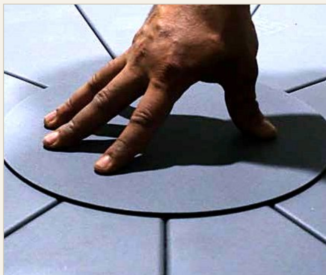
5D-II · HUB COVER PRESSED ONTO ITS SILICONE BED
