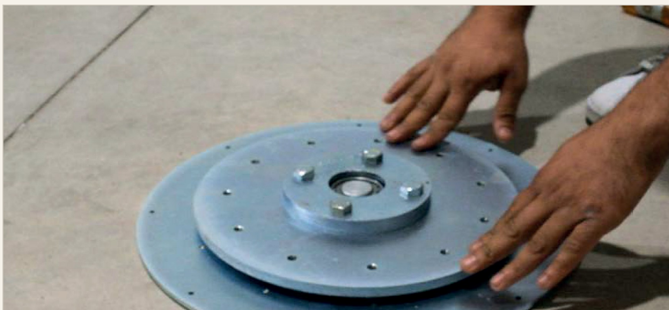
2B · THE UPPER HUB PLATE LOWERED ONTO THE BEARING
