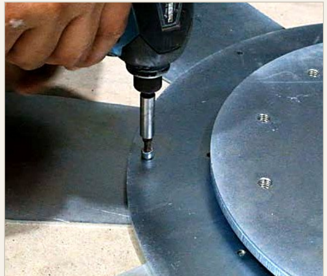
3A · ARMS SECURED BENEATH THE BASE WITH BTR SCREWS
